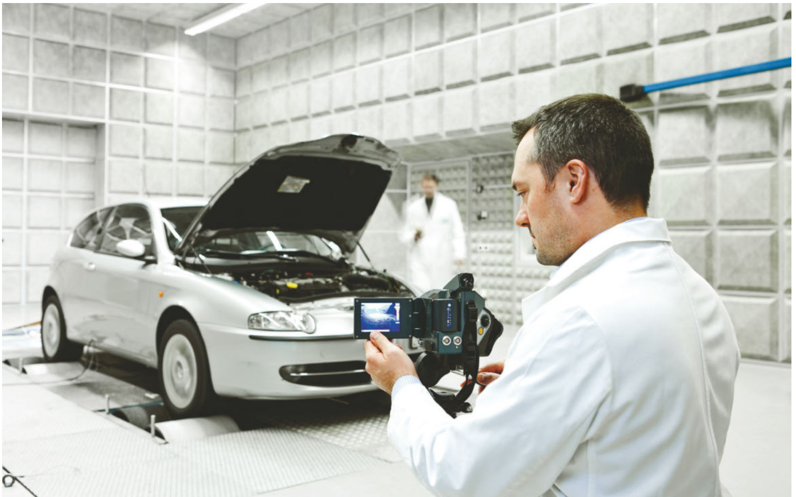
Underbody heat analysis by means of an infrared camera.
